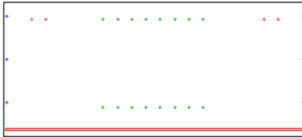
The shelf support holes are in green. The hinge holes are in red. The construction holes are in blue. Here is an example of a 600mm X 768mm lower side panel with a 160mm drawer again using some of the above construction options on the DXF Options page.
