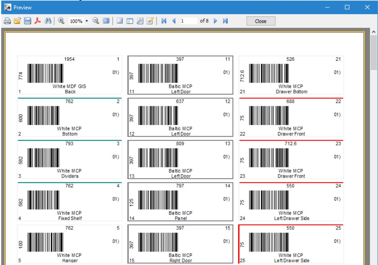
Avery 06498 are removable labels. These labels are 30 per sheet and are removable. The labels print in metric or inches. The width and length are to the left and above the bar code. The top right hand corner has the page number and item number which correlates with the sheet report. This make it easy to determine which label belongs to which sheet.
